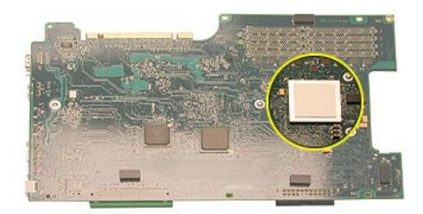
2. Install the replacement logic board in the bottom housing, making sure the board fits over the four mounting pegs on the chassis floor.
